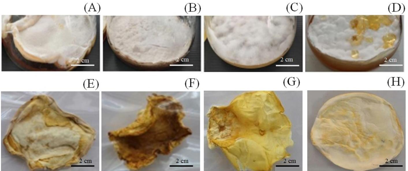
**Figure 1.** Freshly grown mushroom mycelia on the surface of the broth media after 30 days (A-D) and dried mycelium sheets (E-H). The following samples are displayed: LwMEB (A and E), LwPMPB (B and F), OyPDB (C and G), and OyYEB (D and H).
