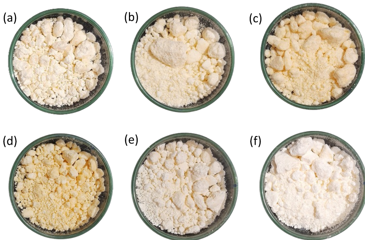
FIGURE 2. Color of nutmeg fat extracted at (a) 300 Watts for 45 min, (b) 300 Watts for 90 min, (c) 300 Watts for 135 min, (d) 450 Watts for 45 min, (e) 450 Watts for 90 min, (f) 450 Watts for 135 min.
