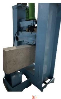
FIGURE 5. Test apparatus. (a) Compressive strength test and (b) Three-point bending test.
