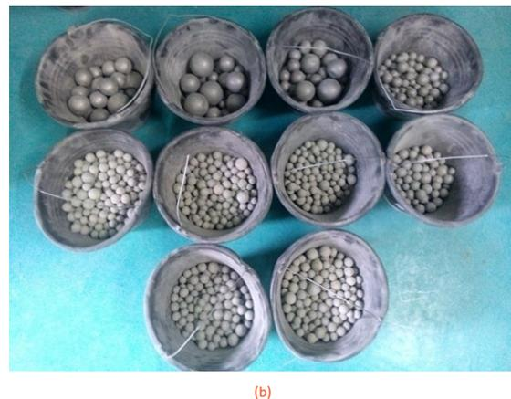
FIGURE 4. Steel ball samples for each chamber of tube mill (a) Chamber 1, and (b) Chamber 2.
