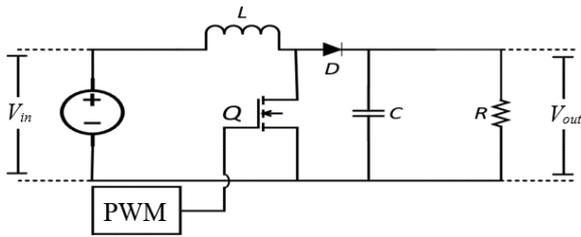
Fig. 1 Basic topology of the boost converter.
