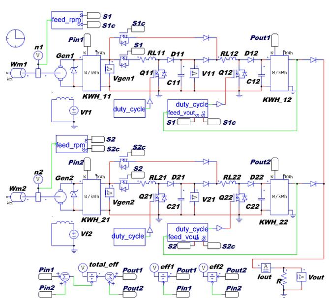
Fig. 8 Simulation circuit of parallel system.
