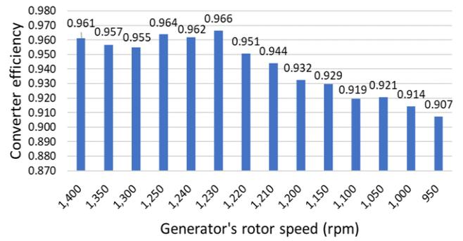
Fig. 12 Simulation result of efficiency of parallel system with same RPM.
