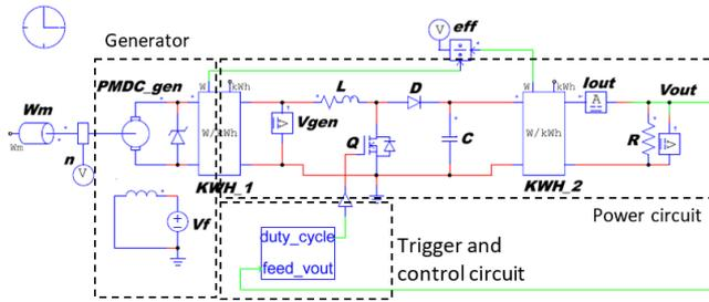
Fig. 5 Simulation circuit of single converter system.
