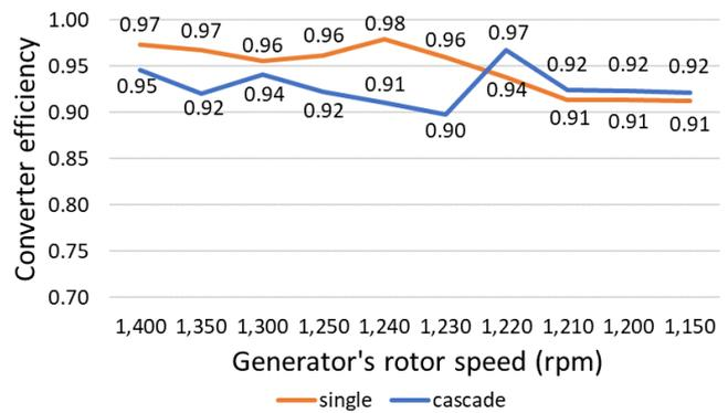
Fig. 10 Simulation result of efficiency of single and cascaded boost converters.
