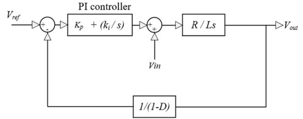
Fig. 2 Closed loop system of boost converter with PI controller [26].
