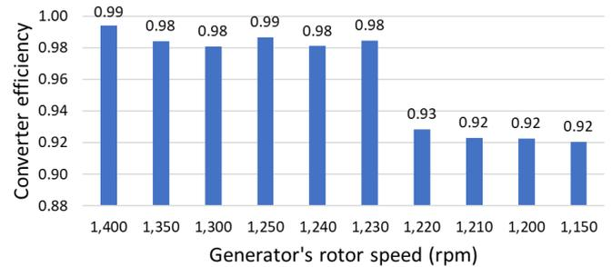
Fig. 11 Simulation results of efficiency of cascaded converters system with selector.
