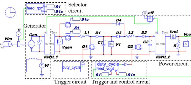
Fig. 7 Simulation circuit of cascaded converters system with a selector.
