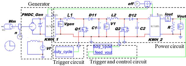
Fig. 6 Simulation circuit of cascaded converters system.
