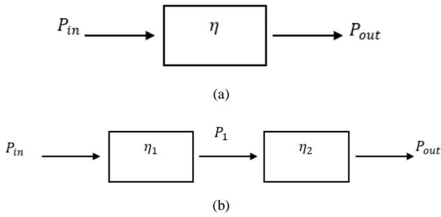
Fig. 3 Efficiency of (a) single device and (b) cascaded devices.
