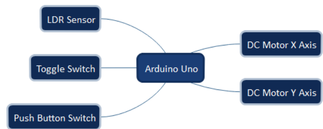
Fig. 1 Block diagram of input and output pin on Arduino Uno.
