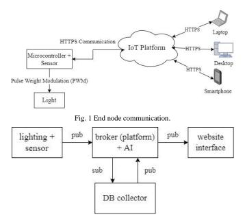
Fig. 2 Data flowchart for smart lighting.
