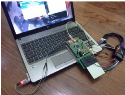
Gbr. 13 Setup eksperimen pengujian smart card reader .
