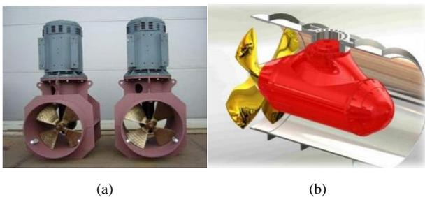
Gbr. 2(a) Motor *gear driven*, (b) Motor *e-pod bow thruster*.
