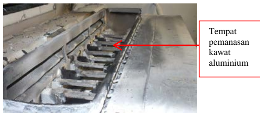
Gbr. 4 Evaporator mesin metallizing .
