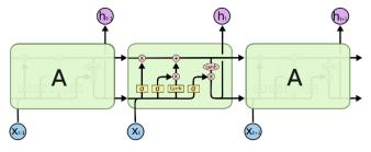
Fig. 1 Four layers of activation functions in LSTM cells.
