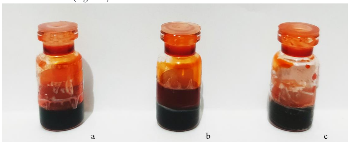
Figure 1. Visual appearance of crude RFO (a), RFO applied to activated carbon treatment (b), and RFO applied to bentonite treatment (c).
