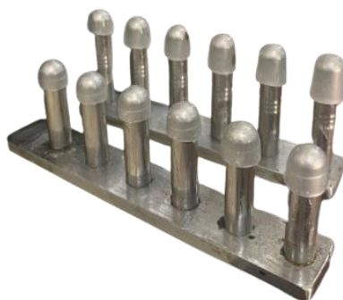
Figure 1. Capsule shell molding process
