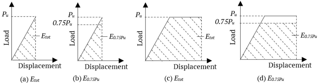
Figure 7 Energy under the load-deflection curve (Spadea et al., 1997)
