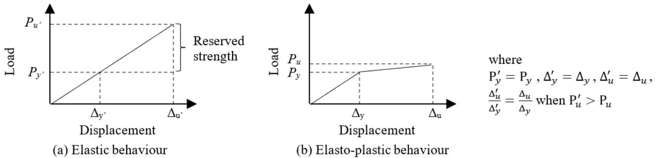
Figure 5 Ductility of the members with elastic and elastoplastic reinforcements
