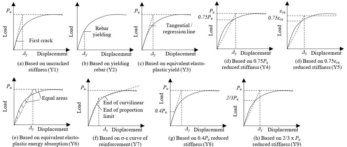
Figure 2 Alternative definitions for yield displacement
