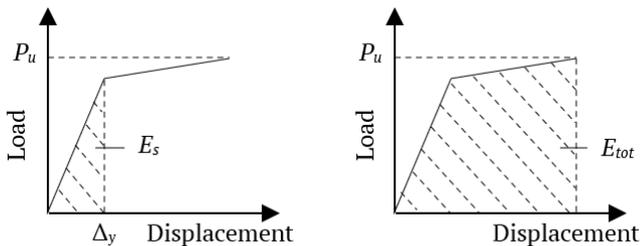
Figure 8 Energy under a load-deflection curve
