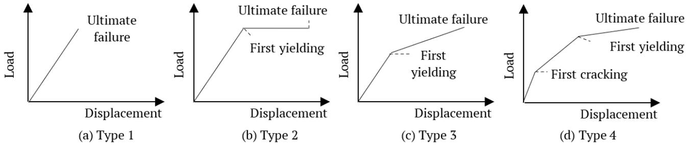
Figure 1 Typical load-displacement curves of structural elements
