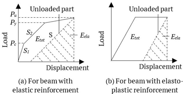
Figure 6 Total and elastic energy under the load-deflection curve (Naaman and Jeong, 1995)
