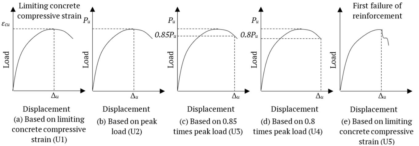
Figure 3 Alternative definitions for ultimate displacement
