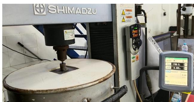
Figure 7 Shear failure test on medium clay soil samples
