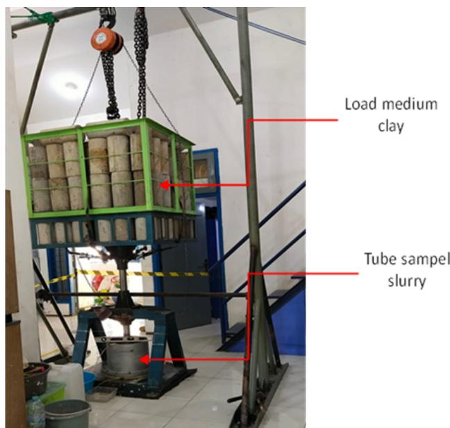
(b) Compression of the slurry sample
