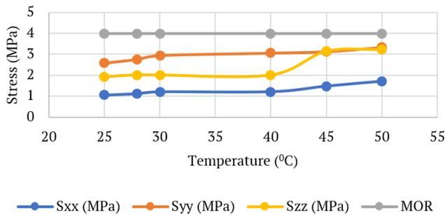
Figure 16 Stress due to temperature variations and edge load position
