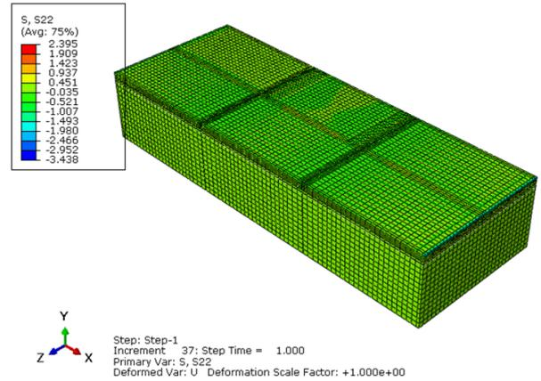
Figure 11 Stress ( $S_{yy}$ ) Contour in Rigid Pavement due to Temperature Load (50°C)
