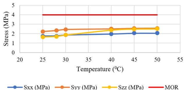
Figure 15 Stress due to temperature variations and corner load position
