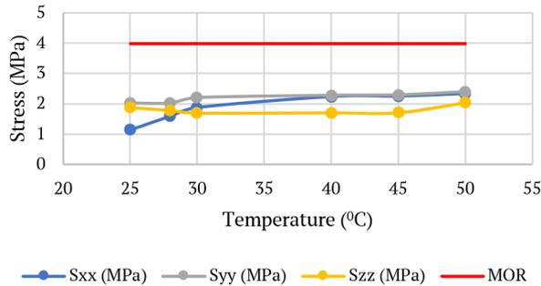
Figure 10 Stress on the influence of temperature on the rigid pavement concrete slab
