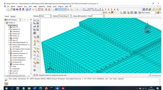
(b) Mesh between slab, sub-base, and subgrade
