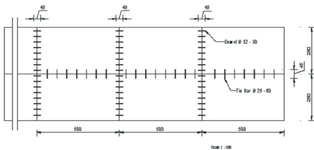
Figure 3 The geometry of the rigid pavement section at Sleman District, Yogyakarta (Scale 1:100)
