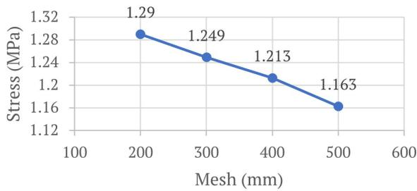
Figure 6 Convergence test on the Rigid Pavement Models
