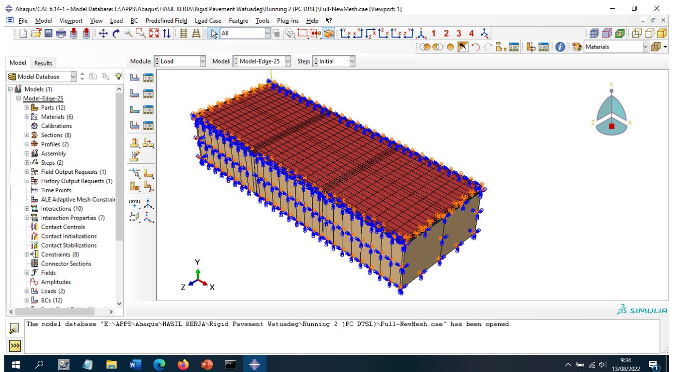
Figure 8 The boundary conditions of the rigid pavement
