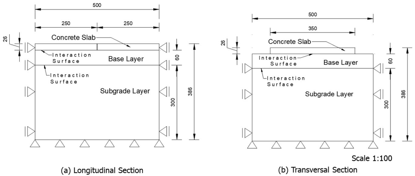
Figure 7 The boundary conditions of the rigid pavement (El-nakib, 2007)
