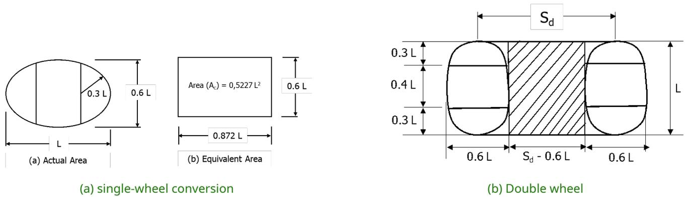
Figure 2 The dimensions of vehicle contact pressure
