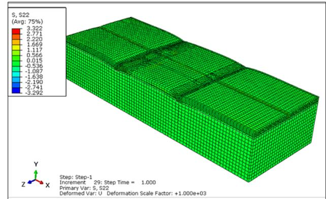
Figure 17 Stress ( $S_{yy}$ ) contour in Rigid Pavement due to combination load (Edge Load + 50°C)
