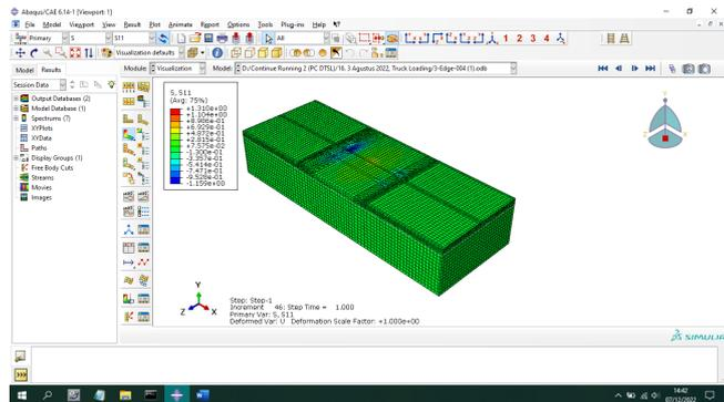
Figure 13 Stress ( $S_{yy}$ ) Contour in Rigid Pavement due to Vehicle Load (50°C)
