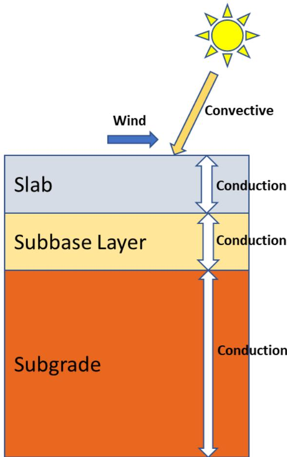
Figure 1 The illustration of heat transfer scheme (Qin and Hiller, 2011)
