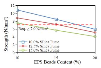
Figure 2. Compressive strength of specimens
