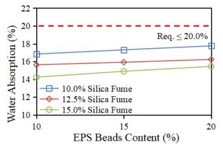
Figure 4. Water absorption of specimen
