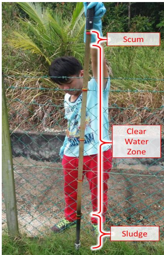
Figure 3. The thicknesses of sludge, clear zone and scum as captured and observed by a sludge judge
