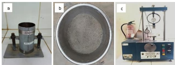
Figure 4. a) UCS mold; b) Specimen mixing bowl; c) UCS testing machine
