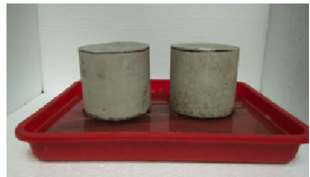
Figure 3. Sorptivity test set-up
