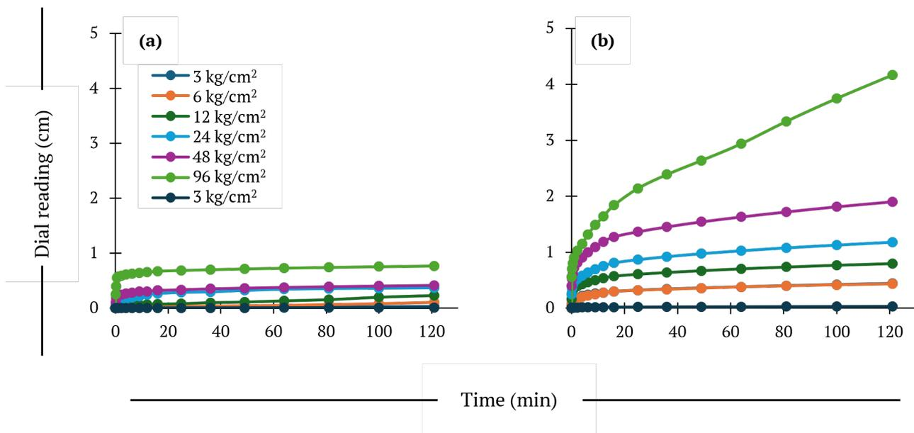
Figure 5 Dial Reading Data for models (a) Without PVD and (b) with PVD
