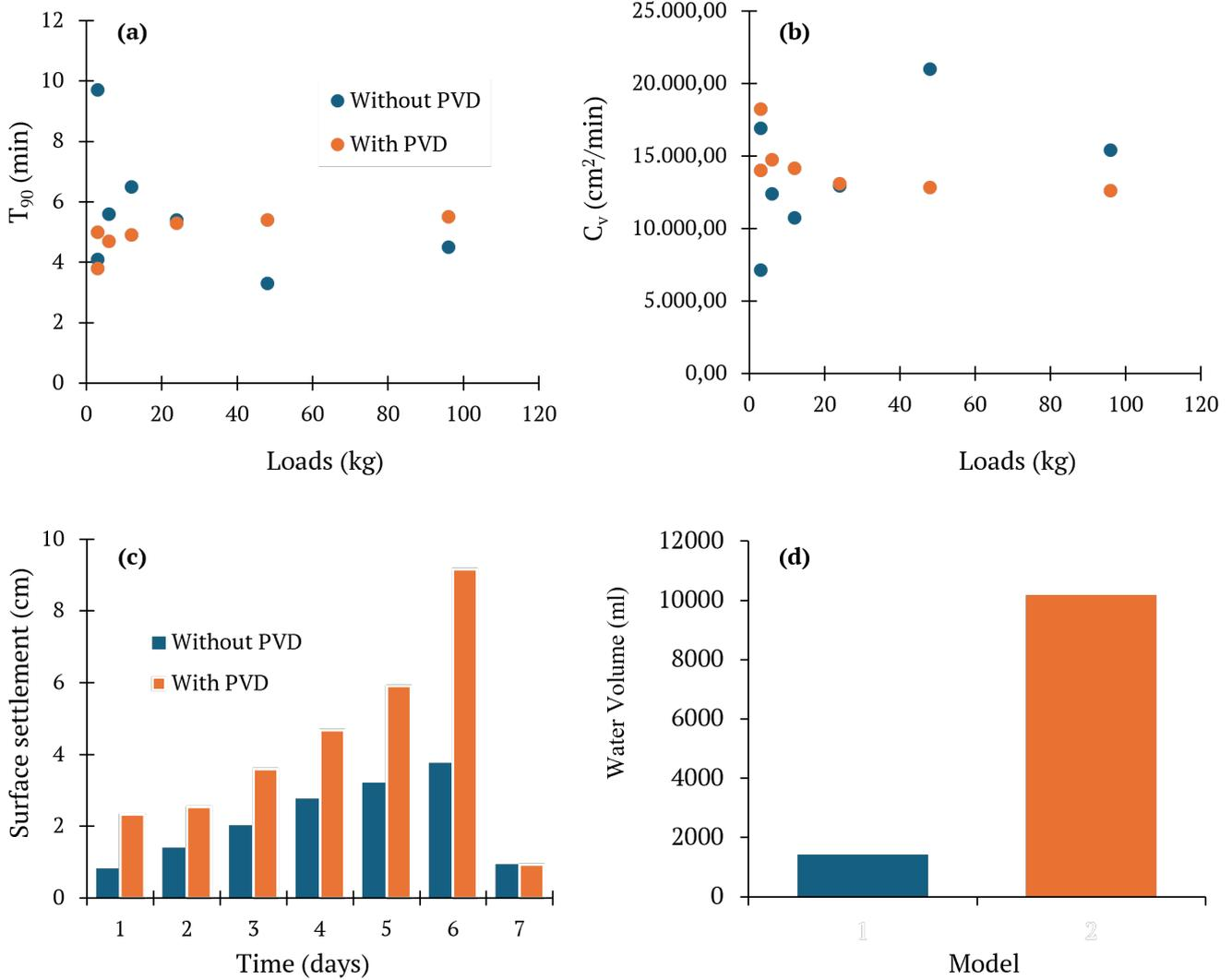
Figure 6 Soil behavior during consolidation process: (a)  $t_{90}$ , (b)  $C_v$ , (c) Surface settlement, and (d) Water discharge.
