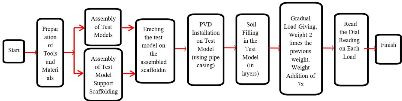
Figure 2 Schematic illustration of the experimental setting
