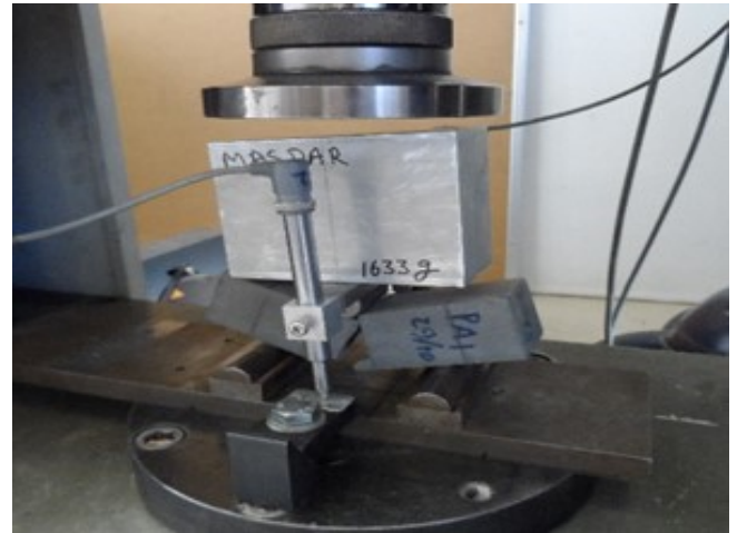
Figure 6 Failure condition of sample after peak load
