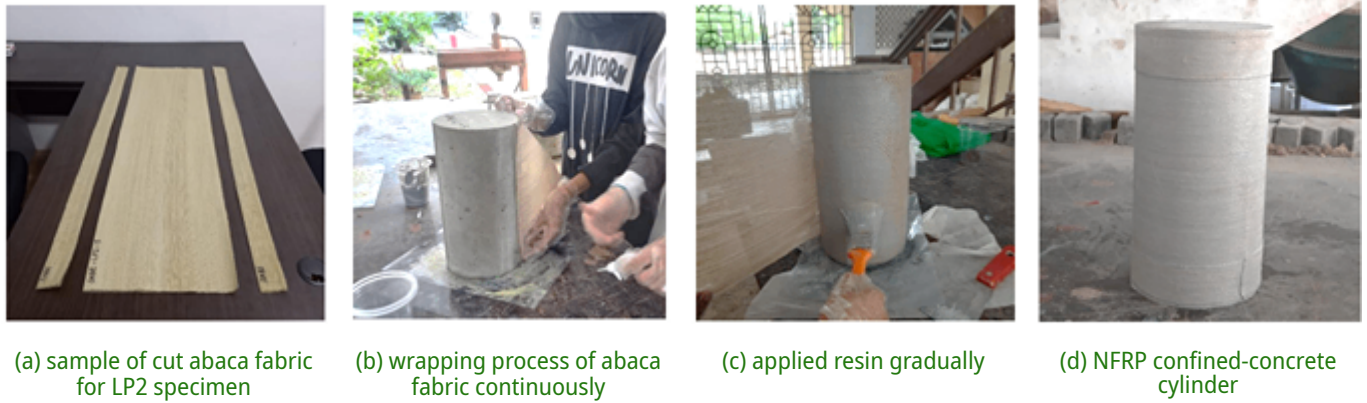
Figure 2 Fabricated NFRP-confined concrete process
