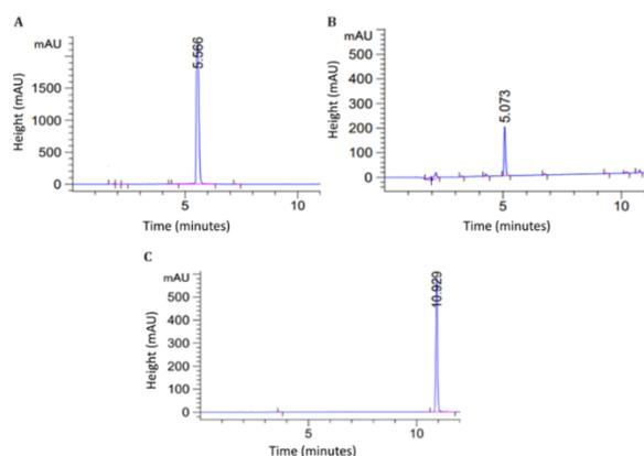
Figure 4. Chromatogram results of antibiotics: a. Ciprofloxacin (CIP); b. Ampicillin (AMP); c. Chloramphenicol (CMP) using diode-array detection (DAD)
