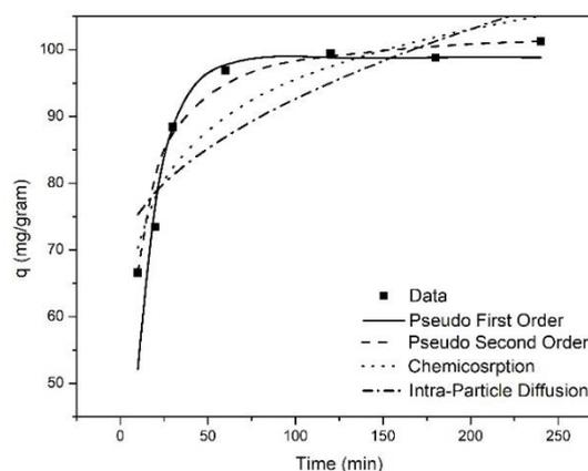
**Fig. 2:** Evaluation of Adsorption Kinetics Model of FFA into Resin
