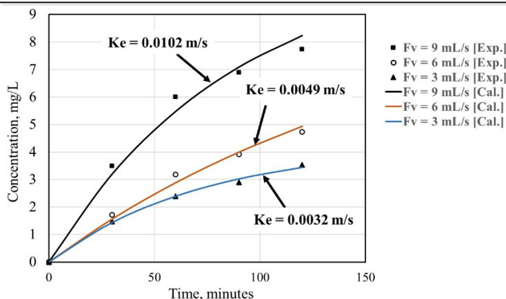
**Fig. 4:** Concentration of flavonoids as a function of time and solvent flow rate based on the calculation and experimental data for the particle diameter of 4.01 mm.
