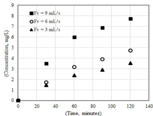
**Fig. 2:** The concentration of flavonoids extracted using different solvent flow rates as a function of time for the particle diameter of 4.01 mm.
