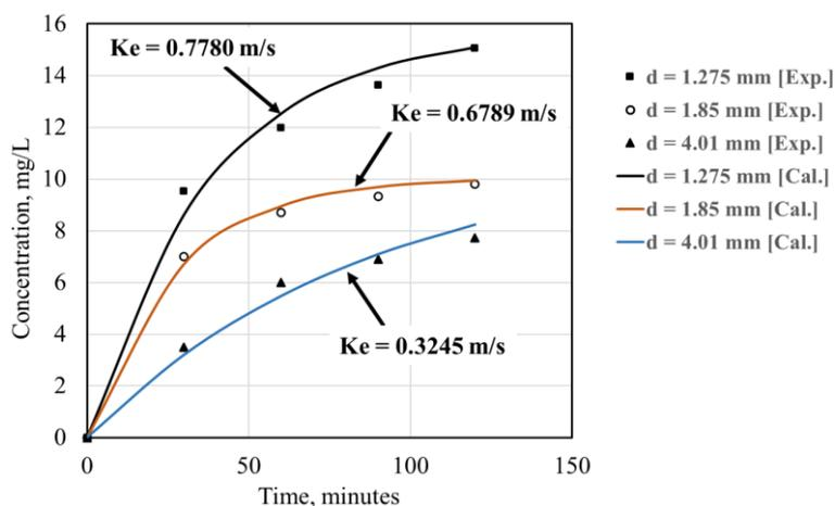
**Fig. 5:** The concentration of flavonoids as a function of time and particle size based on the calculation and experimental data for the solvent flow rate of 9 mL/s.
