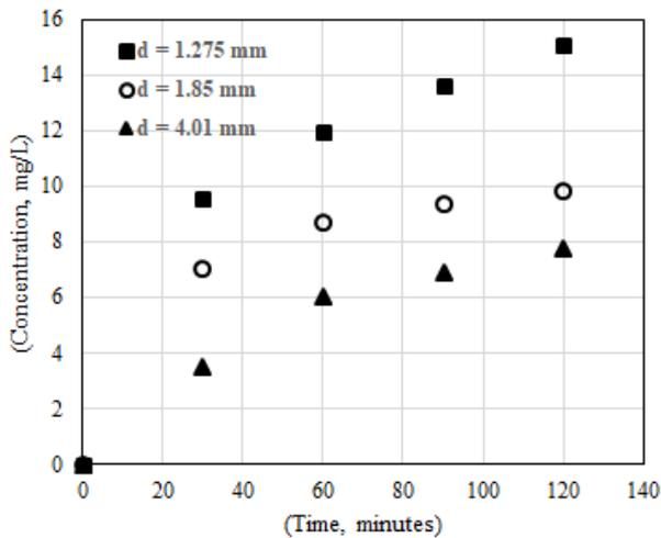
**Fig. 3:** The concentration of flavonoids at different particle sizes as a function of time for the solvent flow rate of 9 mL/s.
