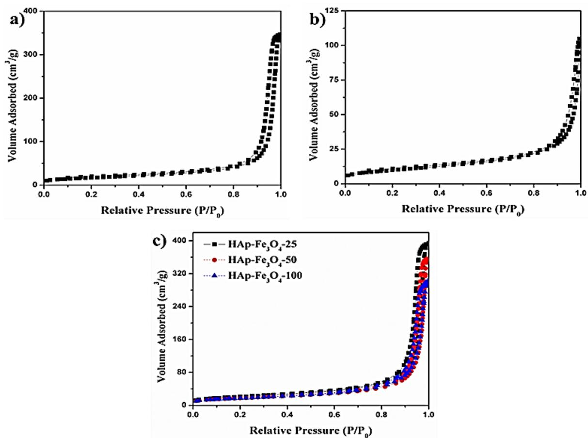
**Fig. 4:** N<sub>2</sub> adsorption-desorption isotherms of a) hydroxyapatite, b) Fe<sub>3</sub>O<sub>4</sub>, and c) HAp-Fe<sub>3</sub>O<sub>4</sub>
