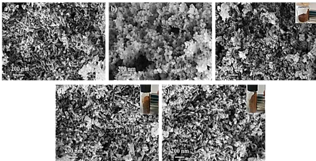
**Fig. 3:** FESEM morphology of a) hydroxyapatite, b) Fe<sub>3</sub>O<sub>4</sub>, c) HAp-Fe<sub>3</sub>O<sub>4</sub>-25, d) HAp-Fe<sub>3</sub>O<sub>4</sub>-50, and e) HAp-Fe<sub>3</sub>O<sub>4</sub>-100.
