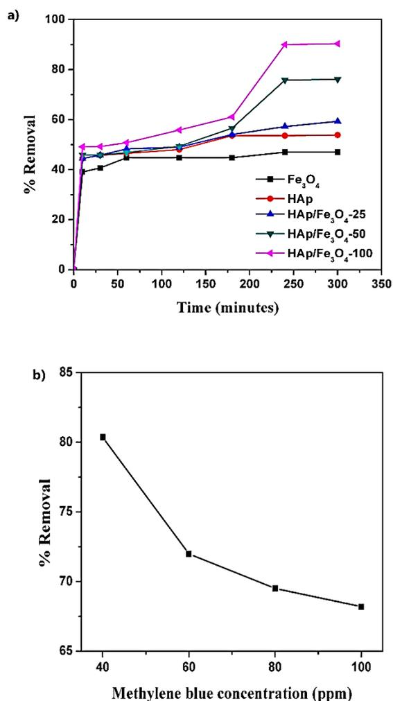
**Fig. 5:** a) Effect of contact time on methylene blue removal by using all adsorbents and b) effect of initial concentration on methylene blue removal by using HAp-Fe<sub>3</sub>O<sub>4</sub>-100
