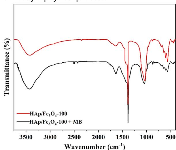
**Fig. 6:** FTIR spectra before and after the adsorption
