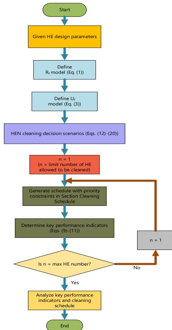
**Fig. 3:** Computation flowchart of cleaning scheduling for HEN
