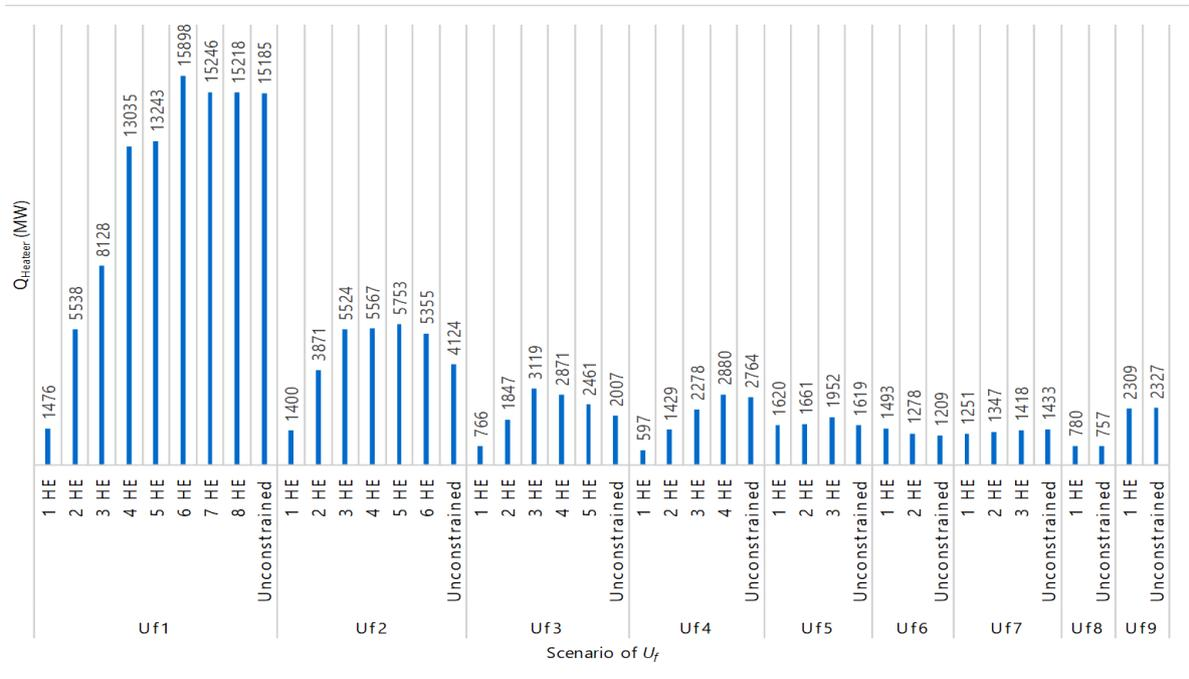
Fig. 5: Heat duty of the heater before desalter in one year
