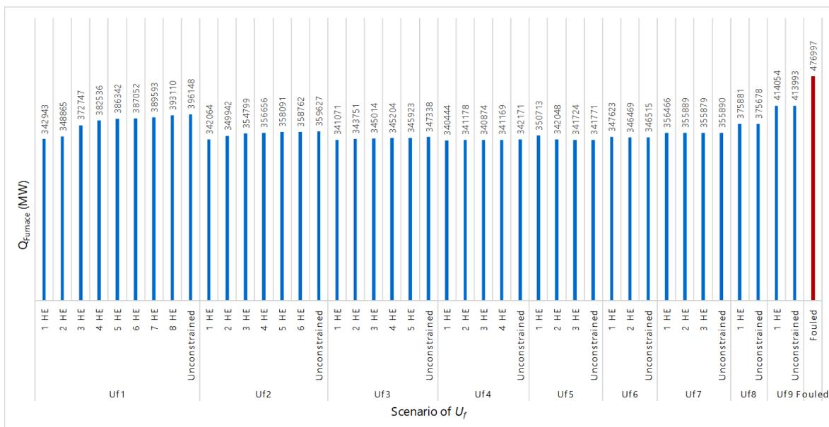
Fig. 6: Heat duty of the furnace in one year
