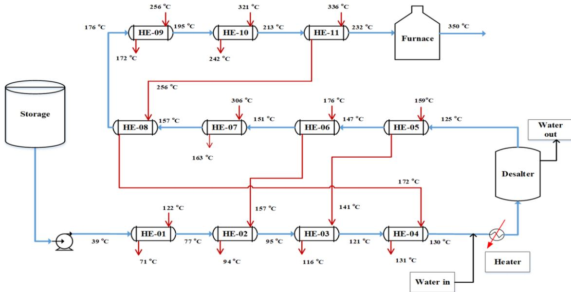
**Fig. 1:** Schematic diagram and typical operating conditions of the HEN in a crude oil refinery (Biyanto et al. 2016)
