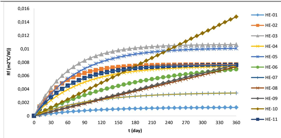
**Fig. 2:** Profile of  $R_f$  for each HE
