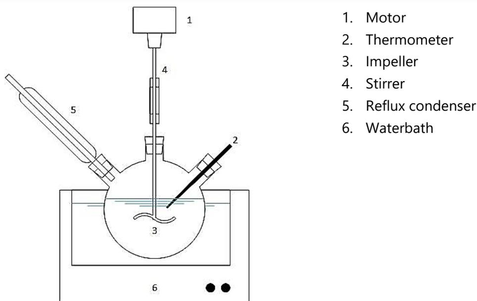
**Fig. 2:** The experimental set-up used for carotenoid extraction
