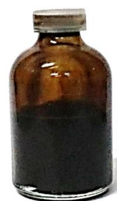
Fig. 8d: Polyglycerol obtained after an 8-hour reaction at 260–270°C with KOH catalyst
