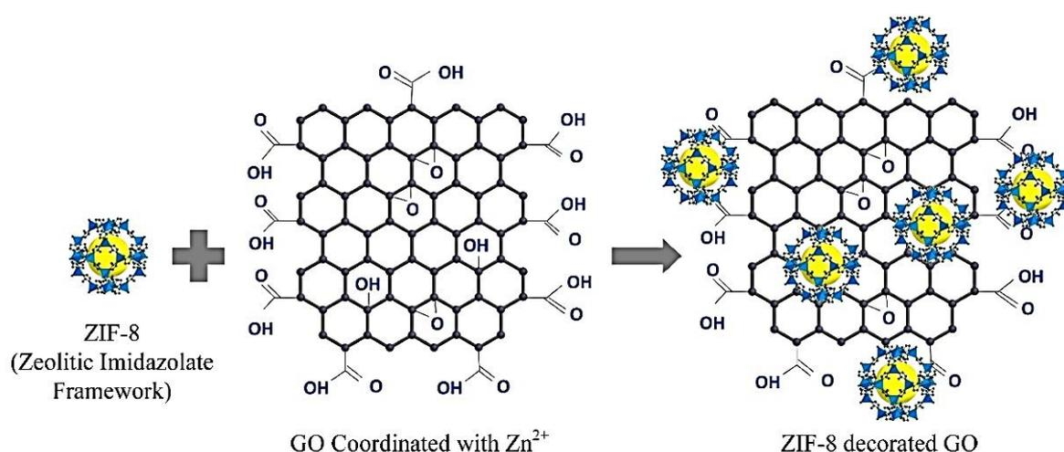
**Fig. 5:** Schematic reaction of ZIF-8 decoration on GO nanosheets (Ahmad et al., 2020)
