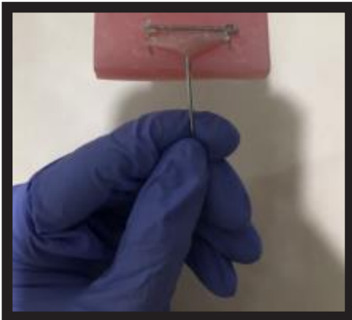
Figure 1. Installation of closed coil springs to acrylic posts with T sticks spaced 25 to avoid deviation
