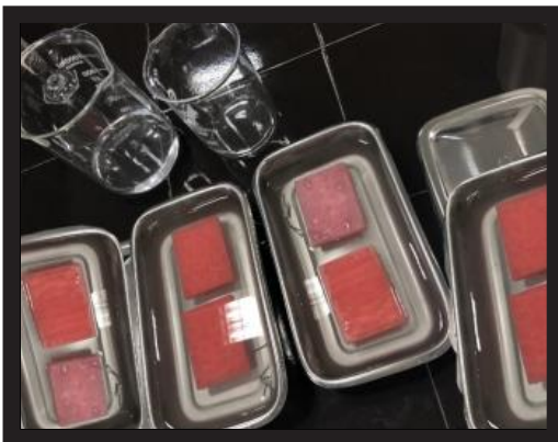
Figure 3. Acrylic block and closed coil spring immersed in a stainless steel filled with artificial saliva
