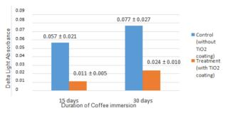
**Figure 4.** The diagram of means and standard deviation of delta light absorbance of control and treatment groups before and after coffee immersion for 15 and 30 days
