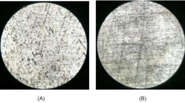
**Figure 5.** Description of thermoplastic nylon surface using a light microscope (Leica, DM 500) 100 times magnification, (A) Control group without  $TiO_2$  coating, (B) Treatment group with  $TiO_2$  coating
