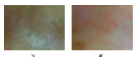
Figure 6. The color of thermoplastic nylon surface after coffee immersion (digital microscope, Dino-Lite, 20 times magnifying) (A) Control group, (B) Treatment group
