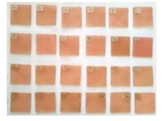
Figure 3. The color of all thermoplastic nylon sample after coffee immersion
