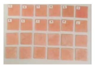
Figure 1. The color of all thermoplastic nylon sample before coffee immersion
