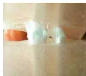
Figure 2. Macro fracture photos on the test rod with the addition of e-glass fiber. Fracture occurs only on resin acrylic.
