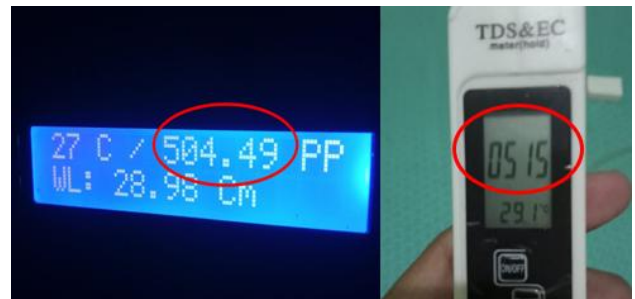
Figure 9. TDS meter sensor calibration result
