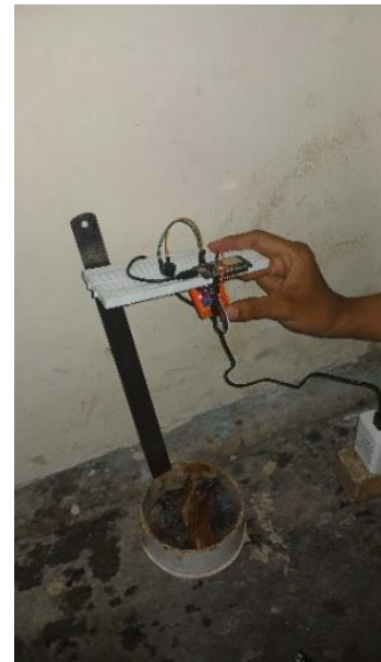
Figure 8. Smoke Sensor Testing Setup
