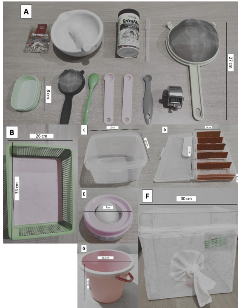
Figure 4. A. Tools and consumables for rearing preadult stage, B. Tray to slow-dry eggs with a cloth, C. Emergence cup for the pupae, D. Container ovicup with the strips, E. Modified sugar cup, F. Customized cage, and G. Bucket for larval rearing.
