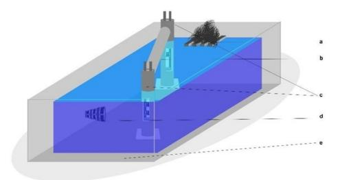
Figure 1. Observation pond design: a. Woven bamboo table, b. PVC pipe to mount the camera, c. Underwater camera, d. Bamboo basket for nesting, e. Breeding pond area.
