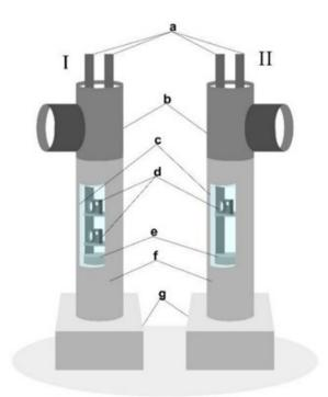
**Figure 2.** Underwater camera design: a. Bamboo stakes for supporting the structure, b. T-shaped PVC pipe fitting, c. 3 mm Acrylic, d. Underwater camera, e. Styrofoam, f. Four-inch PVC pipe, g. Concrete block for support. Camera I is facing toward the nest, and camera II is facing toward the bamboo table.
