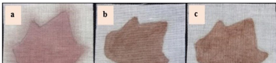
Figure 4. Color tidiness and hue painted with the dye added with additives. The dye (a), the dye + vinegar (b), and the dye + lemon (c).
