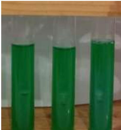
Figure 3. Coliform Confirmation test results on BGLBB Media
