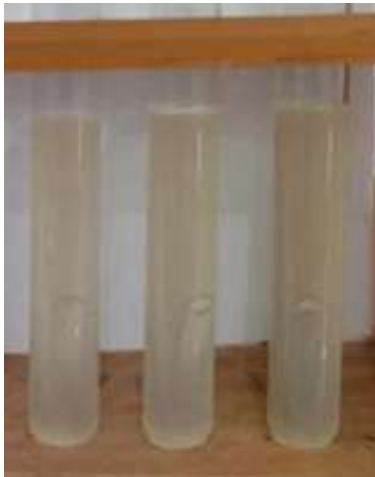
Figure 2. Coliform presumptive test results on Lauryl Sulfate Tryptose Broth (LSTB) Media
