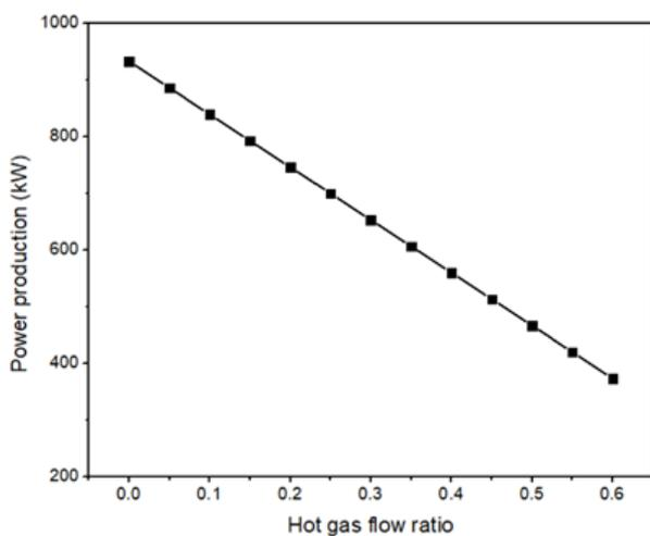
FIGURE 4. Effect of hot gas flow ratio on power production.
