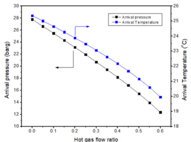
FIGURE 6. Arrival pressure and temperature in process plant at different hot gas flow ratio.
