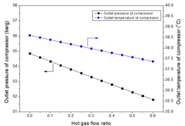
FIGURE 5. Influence of hot gas flow ratio on outlet pressure of compressor.
