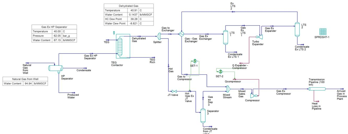
FIGURE 1. Process Flow Diagram (PFD) of dehydration and dew point control unit.
