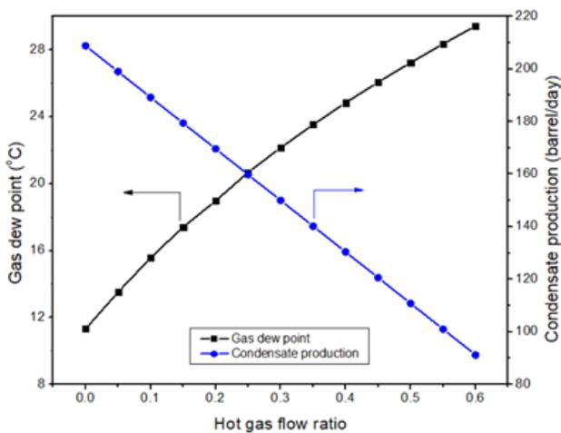
FIGURE 3. Gas dew point and condensate production at different hot gas flow ratio.
