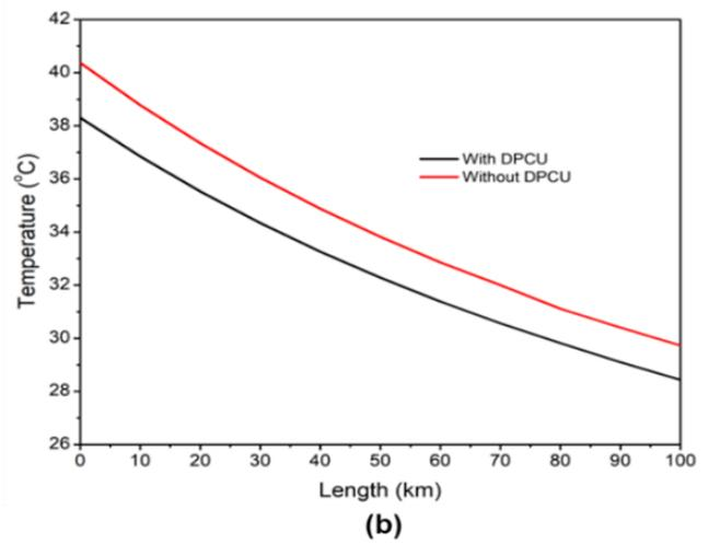
FIGURE 2. (a) Vapor fraction (b) temperature profiles without and with DPCU along pipeline.
