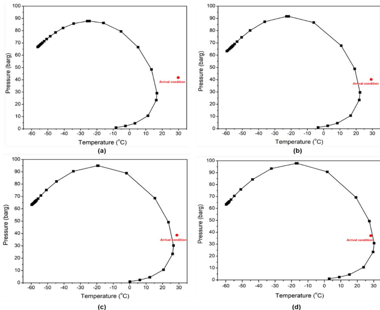
FIGURE 7. Arrival point in dew point curves at hot gas flow ratio (a) 0; (b) 0.2; (c) 0.4; and (d) 0.6.
