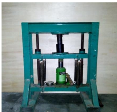
Figure 2. Laboratory-scale pelletizing machine
