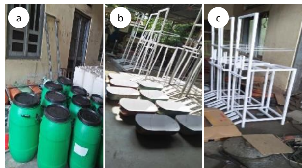
Figure 2 . (a) Water storage material from used drums; (b) Sink material from used Freon tubes that have been painted; (c) Painted sink frame
