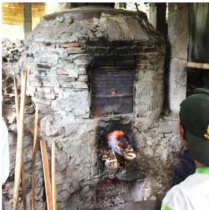
Figure 1. Distiller with a wood furnace in Surya Wulan SME
