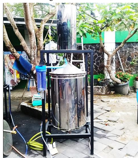
Figure 3. Patchouli oil distiller with a capacity 15 kg of dried patchouli leaves
