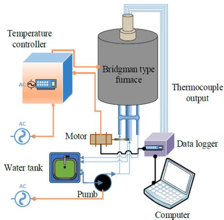
Figure 1. Bridgman-type directional solidification experimental system and equipment
