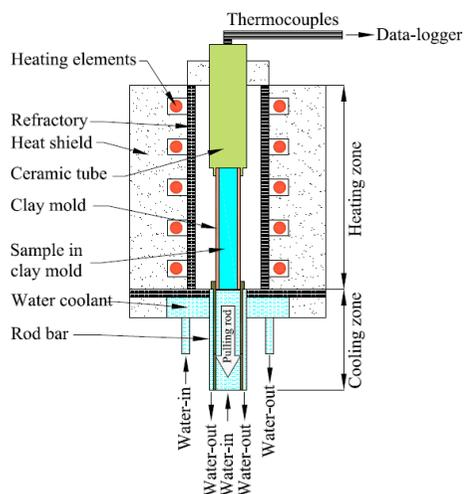
Figure 2. Details of Bridgman-type directional solidification furnace
