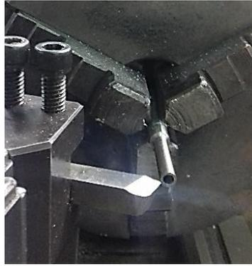
Gambar 2. Proses Face Turning.
