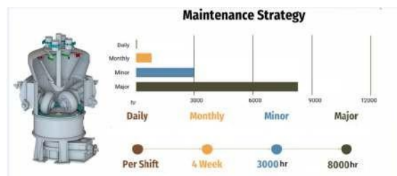
Figure 13. Maintenance strategy for pulverizer mill unit 2E PT PLN Indonesia Power PGU Suralaya
