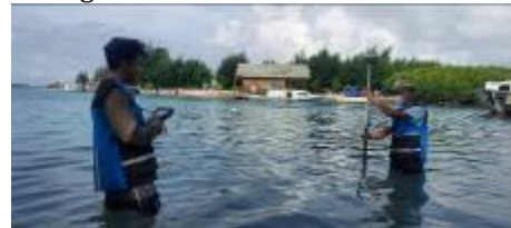
Figure 12 The ICP acquisition at intertidal area
