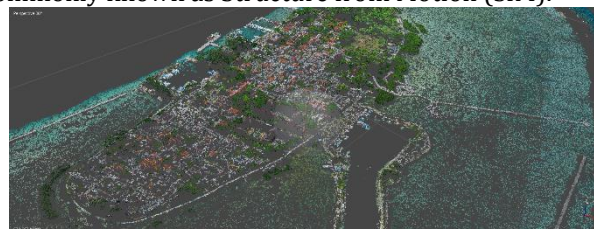
Figure 6 Sparse point cloud at Pramuka Island
