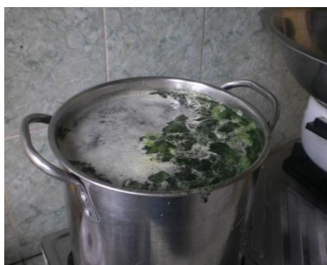
Figure 2. The coagulant (insoluble suji leaf extract) appears in the top of water during suji leave extraction with water as extracting solvent. It contains chlorophyll.
