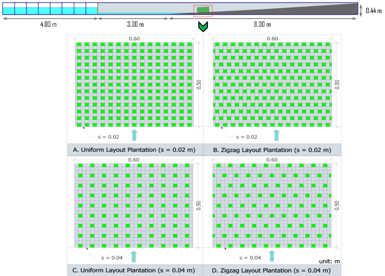
Figure 4. Domain simulation on the flume and the arrangement of uniform and zigzag layout models with variation of spacing between stem ( s )
