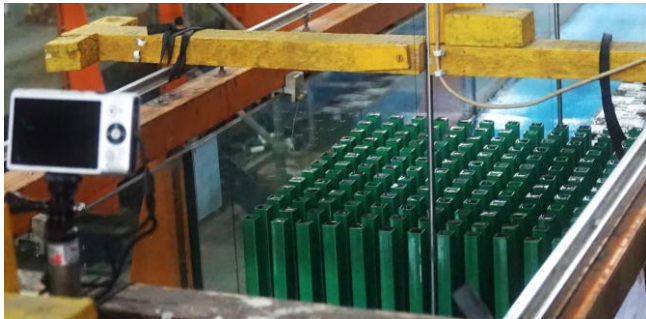
Figure 6. Installation of vegetation model for uniform arrangement type ( s = 0.02 m)
